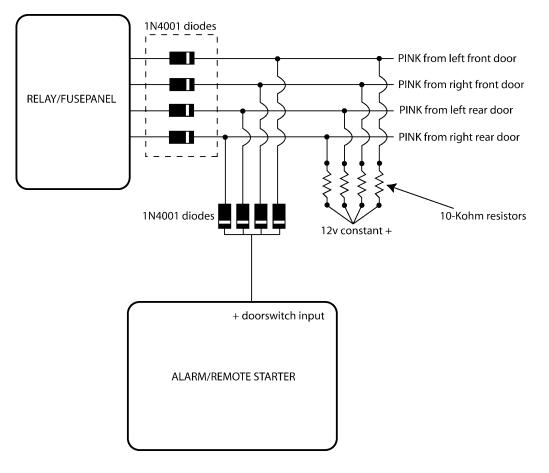
If you are installing a remote start and after-alarm system, you may encounter problems using the courtesy light under the dash as your doorpin input to your alarm system. On a remote start time-out or shutdown, the interior lights on the vehicle come on. This will most likely cause you alarm system to trip. In the event you are using this wire for a manual transmission remote starter, it would take your unit out of ready mode.
